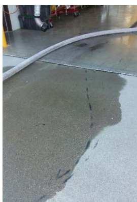
Skid marks caused by hose impact after catastrophic
