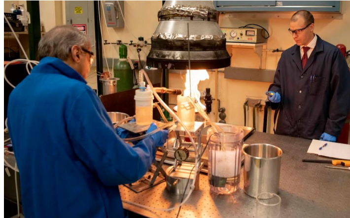
Figure 1 Naval Research Lab Chemical Engineer Gopal Ananth and Research Chemist Spencer Giles test an experimental aqueous film-forming foam at the NRL in Washington, Sept. 23, 2019. NRL scientists are conducting research to support the Defense Department's efforts to replace firefighting foams containing fluorine.
