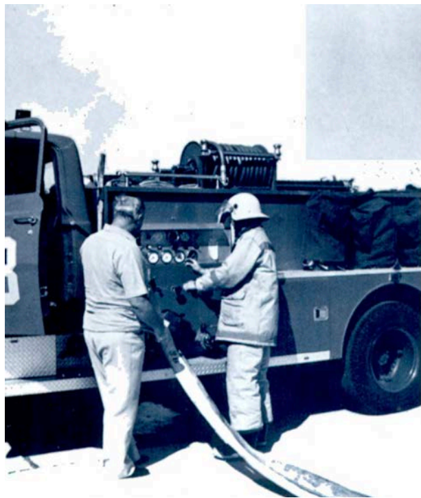
Jerry L. Dallas (left), one of the fire marshals in the Western Division, observes a driver operator as he drafts water off the quay wall at North Island, San Diego, CA.
