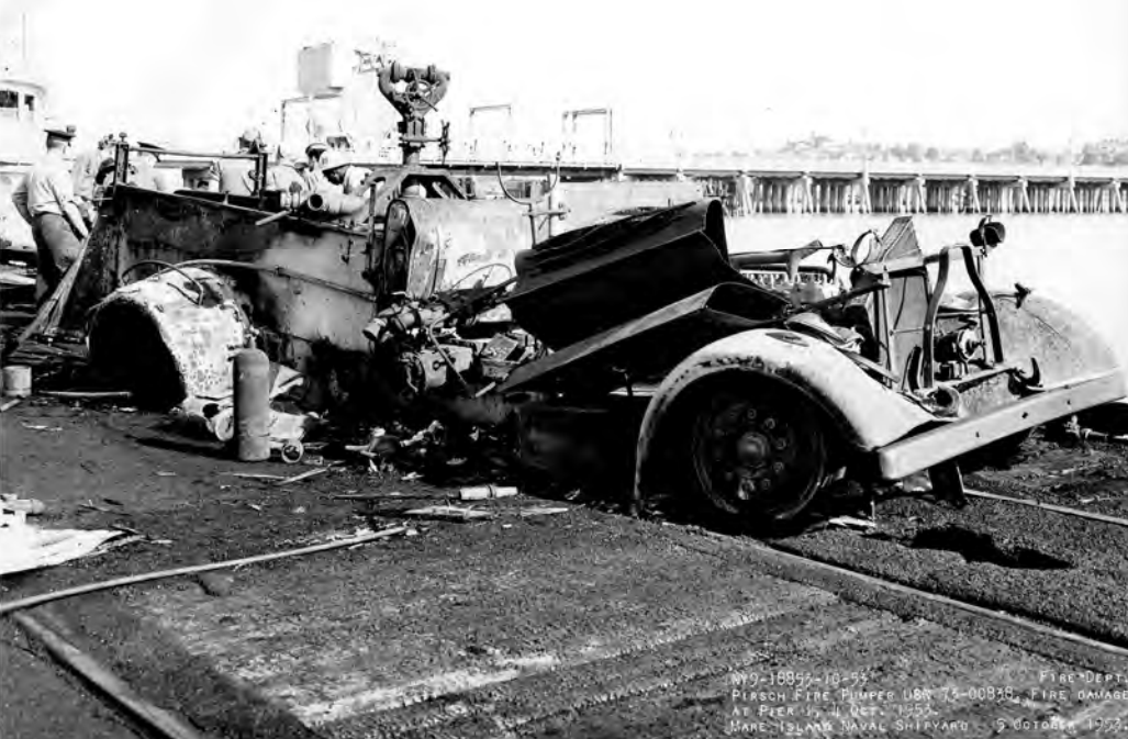
1937 Peter Pirsch pumper, modified with the removal of the top mounted booster reel and replaced with a fixed deck gun. The rig was unfortunately destroyed at a fire on October 4, 1953 which also injured several firefighters.
