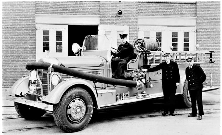
1937 Pirsch Model 25R pumper, 1,000gpm/100gal, Navy property number 73-00838 prior to replacement of top-mounted booster reel.
