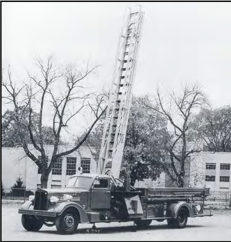
(above) Advance Base Depot 1939 Maxim 65 foot aerial ladder. (bottom) Philadelphia Naval Shipyard 1941 American LaFrance JOX 100 foot aerial ladder.
