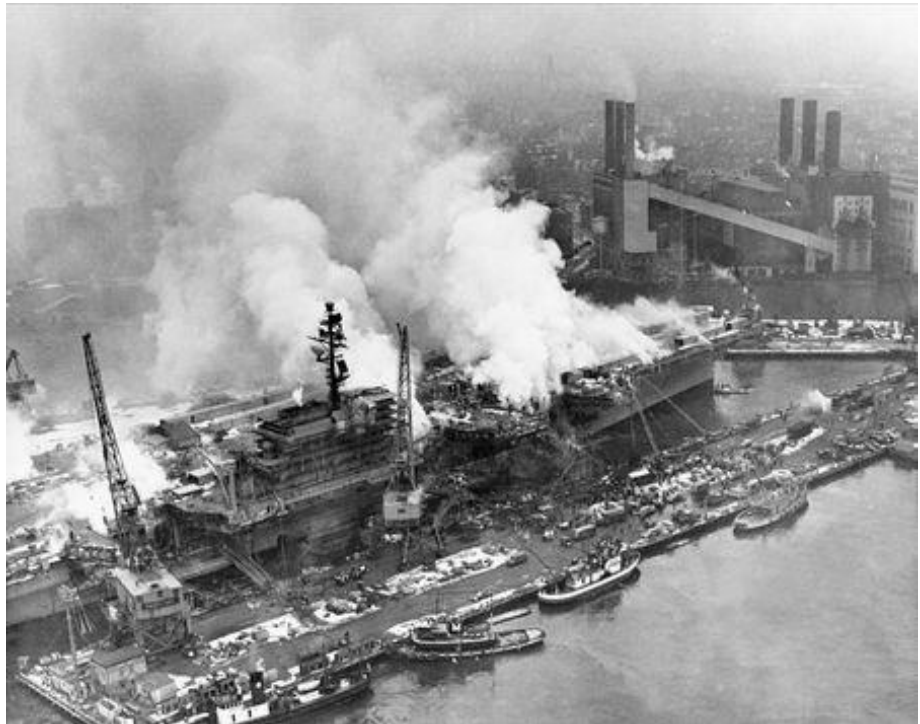
Smoke rises from the fire aboard the navy aircraft carrier USS Constellation at the Brooklyn Navy Yard on the East River in New York, Dec. 19, 1960. In the background is part of the Brooklyn waterfront. The fire began after a forklift collided with fuel tank as construction of the carrier neared completion. Fifty people were killed and hundreds injured. (AP Photo) AP
