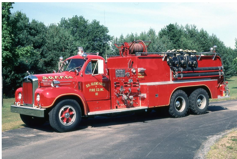
Glens Falls Engine 1959 Mack B-85F 1000 gpm 1500 gwt X-US Navy – provided by Tom Shand
