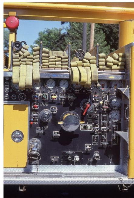
In 1975 the Syracuse, NY Fire Department ordered seven 2000 gpm pumpers from Pierce Manufacturing which would be powered by Detroit Diesel 8V-92TA engines rated at 380 horsepower. These units were among the first Waterous pumps rated at 2000 gpm that were to be equipped with an electronic pressure governor and required both the pump governor and Ross relief valve to pass all of the required UL testing for pump certification.
