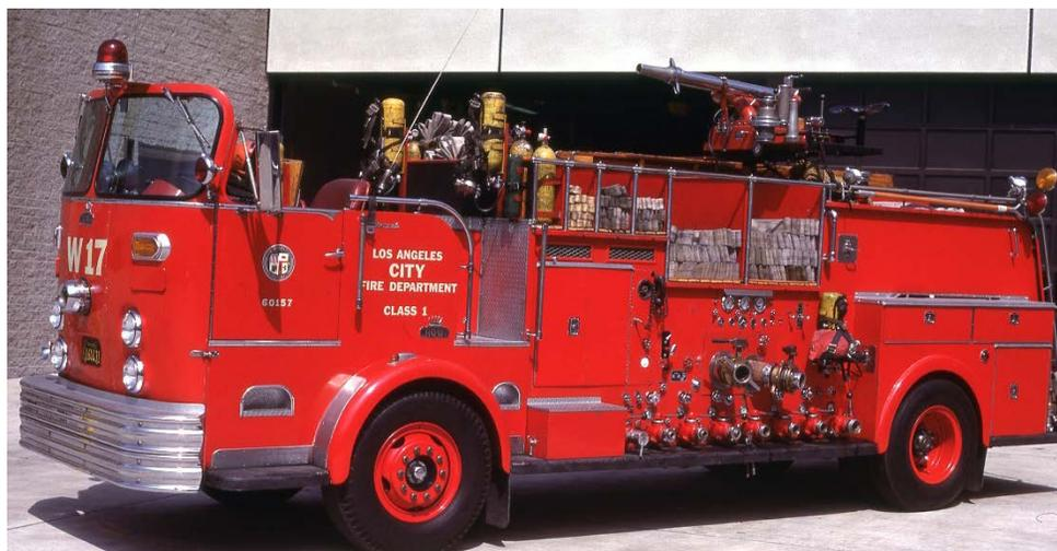
Fire pump technology and engineering enhancements are linked to advancements in engine performance with horsepower and torque ratings. Early motorized pumpers were commonly outfitted with 400 to 600 gpm rated fire pumps due to gasoline engine ratings available in commercial chassis. As apparatus manufacturers began to develop their own custom-built chassis engine horsepower ratings enabled 750 to 1000 gpm two-stage fire pumps to become more prevalent.
