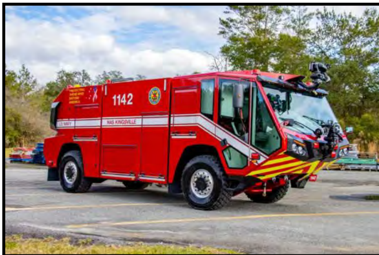
The reduced size TITAN ARFF truck has a Darley PSP 1,500-gpm pump, a 140-gallon polypropylene foam tank, and a 1,000-gallon polypropylene water tank instead of the 1,500-gallon water tank typical on a TITAN ARFF 4×4 AT.
