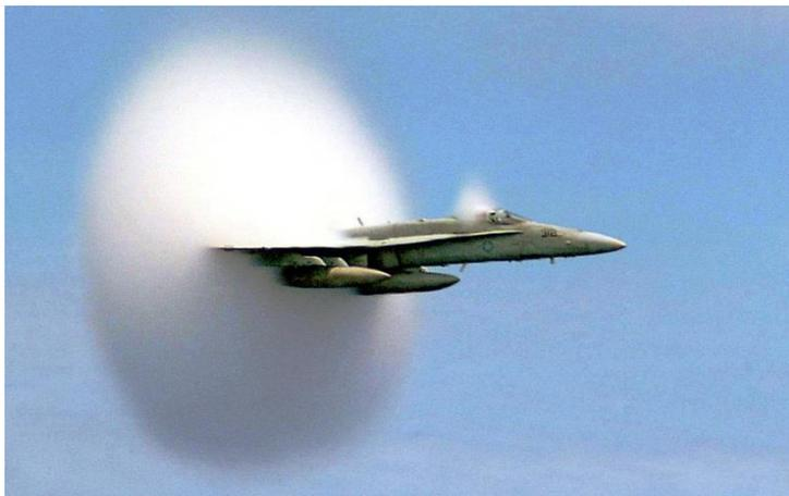
**Above:** F/A-18 Super Hornet approaches the speed of sound. The lens-shaped cloud is condensed water vapor that forms in the area of low pressure. The high-pressure area, or ridge, streams invisibly from the nose and wings of the aircraft.
