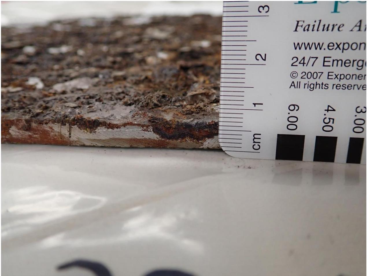
Figure 1: Edge of Coupon #7. Image from non-Navy source alleging the thickness of the remaining steel at the location shown alleging thickness less than the Navy's predictions.
