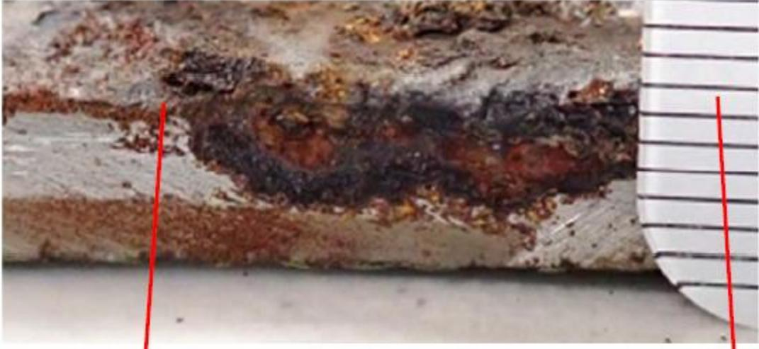
Figure 2: Image taken after coupon removal, prior to receipt by lab. What appears to be a deep corrosion pit was actually rust-covered staining of the edge surface.
